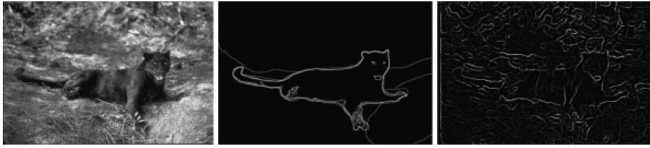
Figure 1. An example from Martin, Fowlkes, and Malik (2004) to highlight the difficulties of bottom-up segmentation. For the image shown on the left, humans see the definite boundaries shown in white in the middle image. The best machine segmentation of a set of algorithms gives the result shown on the right—a mess. This seems a very difficult scene to segment without having some training at least for the specific kinds of materials in the scene.
