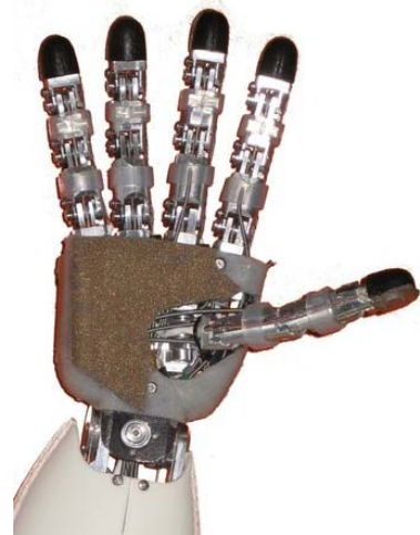
Figure 2: The hand of the iCub , showing some of the tendons, the sensorized fingertips and the coating of the sensors of the palm (108 taxels overall). Tendons are made of Teflon-coated cables sliding inside Teflon coated flexible steel tubes.
