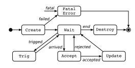
Fig. 3. The life cycle of the Port Monitor Object.
