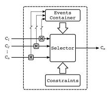
Fig. 5. The architecture of Port Arbitrator object. Straight lines show the data flow and zigzag lines represent event flow.
