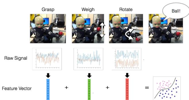
Fig. 1. Object recognition pipeline: (Top) iCub performs different exploratory procedures while holding an object. (middle) the raw sensory signal is coded into feature vectors (bottom) which are used to train haptic classifiers.
