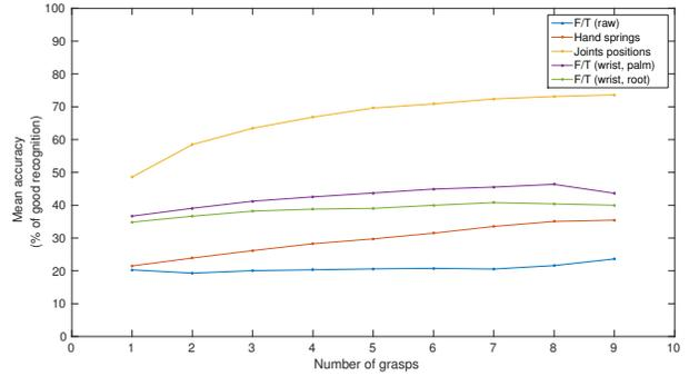
Fig. 8. Evolution of the mean accuracy achieved by combining predictions from 1 to 9 session for each modality separately, with the Grasp EP and the snapshot feature.
