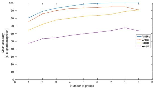
Fig. 9. Evolution of the mean accuracy achieved by combining predictions from 1 to 9 session for each EP separately or all together.
