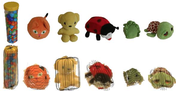
Fig. 9. Top: the objects used in the experiments. Bottom: reconstructed point clouds with superimposed superquadric models.
