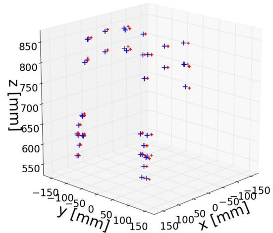
Fig. 13: The red points represent the measured position of the marker. The blue points represent the desired position. The average accuracy is within 11 [mm].
