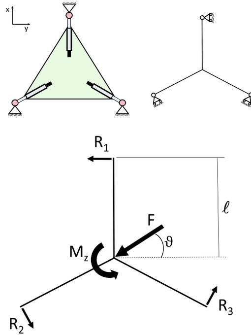
Fig. 5: The top left image represents a 2D model of the platform. The top right image represents the equivalent model, while the bottom image represents its free body diagram.
