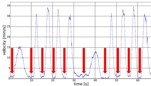
Fig. 10: The average velocity of the chest during one cycle. The peak chest velocity is 35 [mm/s]. During each cycle the platform has been stopped for a few seconds in 10 different poses (red arrows). For each pose we evaluated the repeatability (Figure 11) and accuracy (Figure 13).
