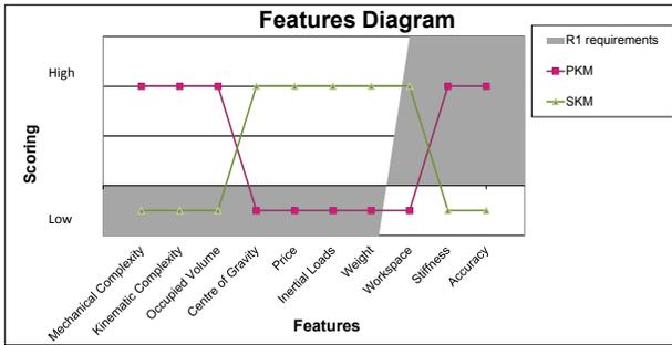
Fig. 2: The diagram compares the serial and parallel manipulators against our design requirements. The features are ordered from left to right to simplify the visualization of the curves minimizing the crossings.
