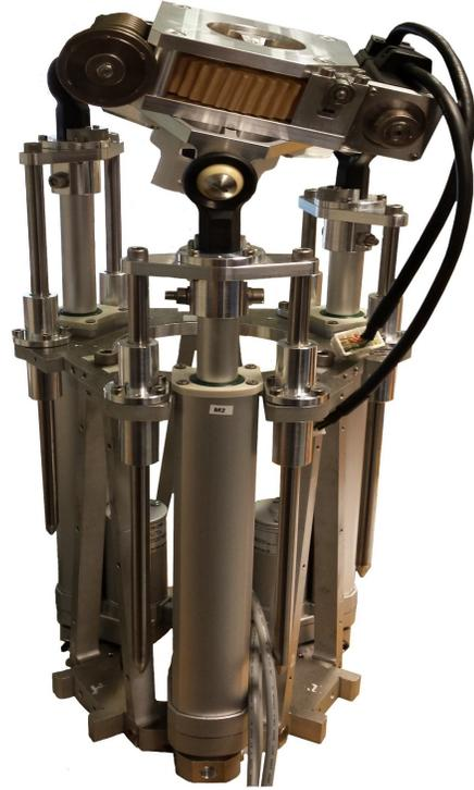
Fig. 1: The figure shows a photograph of the prototype of the torso joint of R1. The system is directly assembled on the mobile base, while the robot chest is connected to the aluminum platform on top of the plastic gear.
