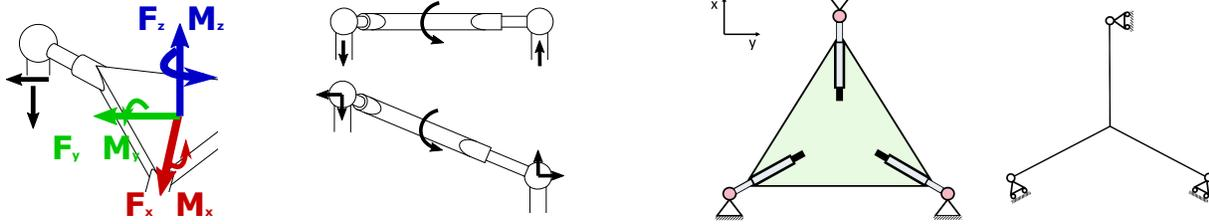
Fig. 4: The left figure: the spherical joints don't produce any reaction moment on the actuator rods. Thanks to this decoupling the only forces acting on the rods are either pure axial loads or radial loads. The right figure: if the platform is horizontal a moment applied to the platform generates pure axial forces on the actuator rods, contrary when the platform is tilted a moment generates also radial forces.
