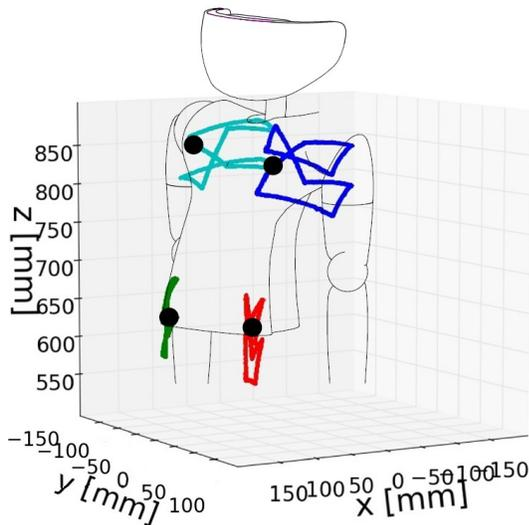
Fig. 9: The four markers have been fixed at two different heights on the chest of R1. For each marker is also plotted the trajectory measured by the motion capture system.
