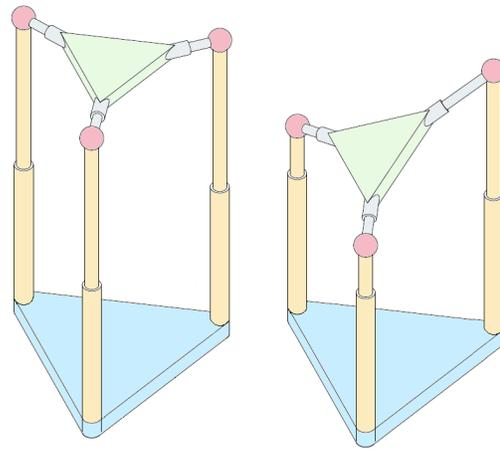
Fig. 3: The conceptual design of the parallel structure in two different configurations. The colors identify the core components of the system: in blue the base, in yellow the linear actuators, in red the passive spherical joints, in gray the passive prismatic joints and in green the platform. When the platform is tilted its center moves also in the horizontal plane.
