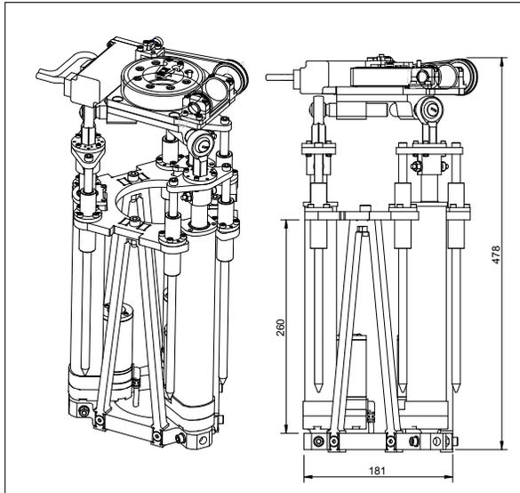
Fig. 6: The final layout of the torso joint. The figure shows the main dimensions of the system.
