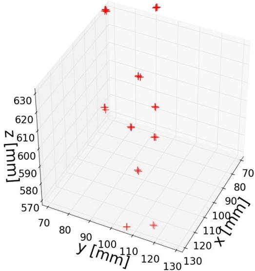
Fig. 12: The points represent the overlapping measurement for one chest marker. The repeatability for this marker is within 2.5 [mm].
