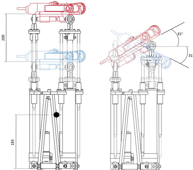
Fig. 7: On the left the heave workspace is depicted by superimposing the fully extended (red) configuration over the fully retracted (blue) configuration. Furthermore the position of the CoM computed for the fully retracted configuration is shown by the black point. On the right the roll (or equivalently, the pitch) workspace is depicted by superimposing the maximum positive and negative platform inclination.
