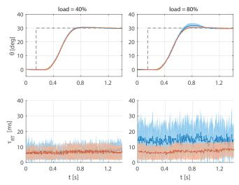
Fig. 7: Evaluation of the joint velocity control experiment. Both system step responses  $\theta$  and round-trip time  $\tau_{RT}$  are depicted in the case of 40% (left) and 80% (right) network loads. The responses corresponding to the use of QoS are in red, whereas the system responses without channel prioritization are in blue. Results are reported in terms of average and confidence interval of 95%.
