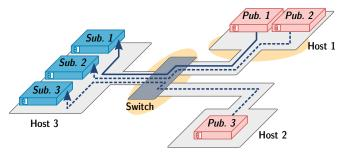
Fig. 4: An example of publish/subscribe architecture in a LAN network consisting of three nodes (Host1, Host2 and Host3) connected through an Ethernet switch. The arrows represent data–flow from publishers to subscribers.
