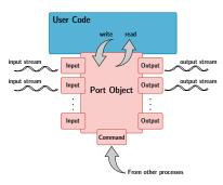
Fig. 2: The internal structure of a YARP port object.
