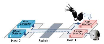
Fig. 1: An example of distributed control architecture in a network consisting of two nodes (Host1, Host2). The arrows represent communication and the data–flow between components.
