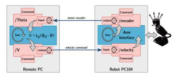
Fig. 6: The velocity control loop.
