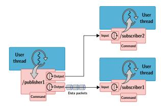
Fig. 3: An example of components asynchronous communication in YARP. A publisher is pushing messages to two different subscribers using separate dedicated threads.
