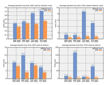
Fig. 5: Evaluation results of channel prioritization at the network card and switch for different loads and transport protocols. The bars labeled as "qos" represent the test results in presence of channel prioritization. The bars labeled as "normal" represent the test results in absence of any prioritization. The number above the bars represent the standard deviations of samples.
